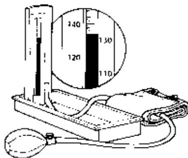
Figure 26.7 A mercury sphygmomanometer – for measuring blood pressure.
