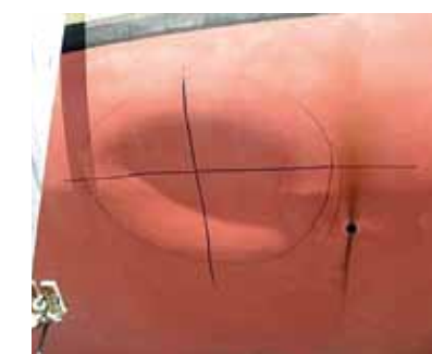
▲ Above: dent in the steel hull of a yacht reportedly made by a sperm whale that attacked the vessel
