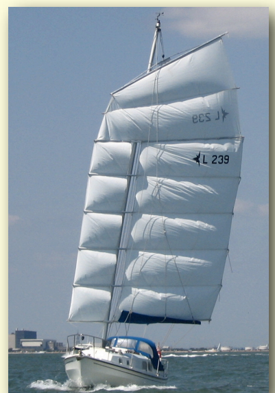
"Poppy", with a 'split junk' rig. Just one example of recent junk rig innovation - windward performance without losing the rig's advantages.
