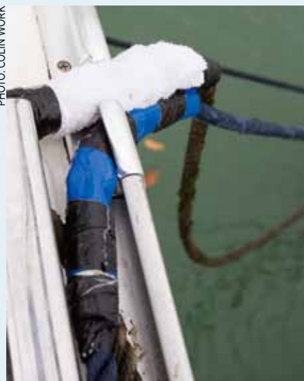
Use your heaviest mooring lines and protect them at any potential chafe points
