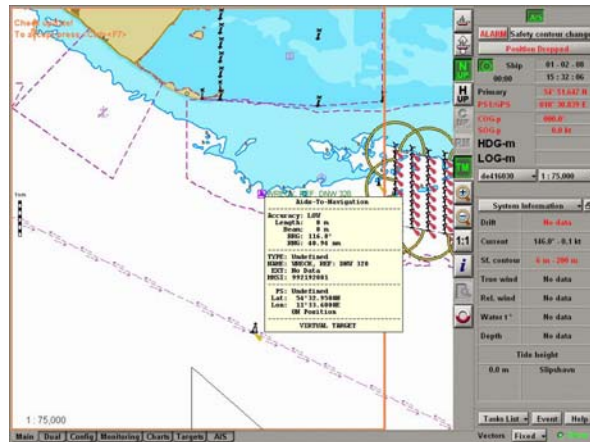
This display system showed the AIS AtoN target, but only after we increased the transmission frequency
