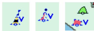
DaMSA proposal regarding symbols for virtual AIS AtoNs, that indicate the type of AtoN
