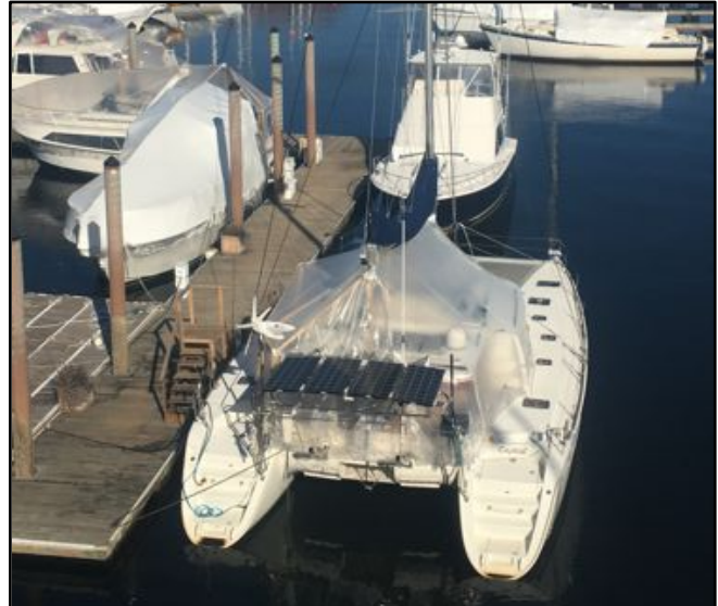
Catamaran using both solar panels and a wind generator for energy.
