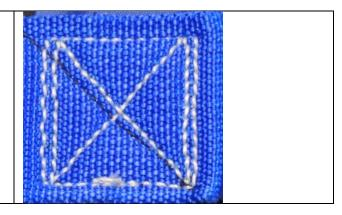
The sewing should be done with a contrasting color thread, to more quickly spot chafe and popped stitches, and triple-stitched using 'machine lockstitches' (the most common sewing machine stitch) so that the stitches are as even as possible in tension and will not quickly unravel if one stitch breaks.
