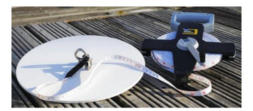
Attached to a measuring tape, the Secchi Disk is lowered over the side of a boat and the depth at which it disappears from sight estimates the amount of phytoplankton in the sea. This depth can then be uploaded to a database using the Secchi app.
