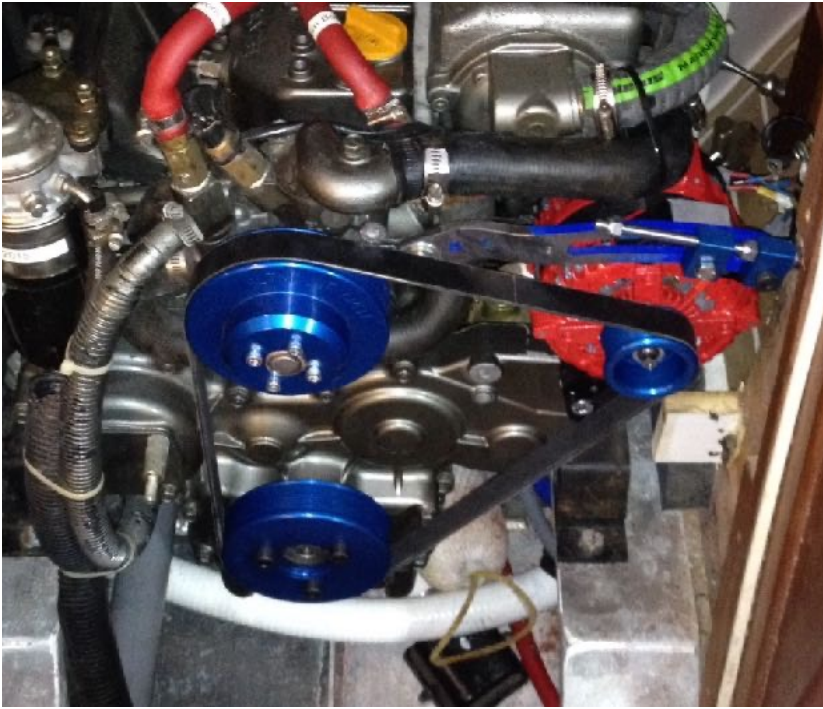
Fig. 5: Balmar alternator (red, 12 V/200 A) with new belt pulleys for flat multigroove belts (blue) and tensioning device (also blue)
