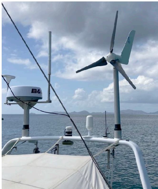
Fig. 4 Wind generator on the gantry (stern bar)
