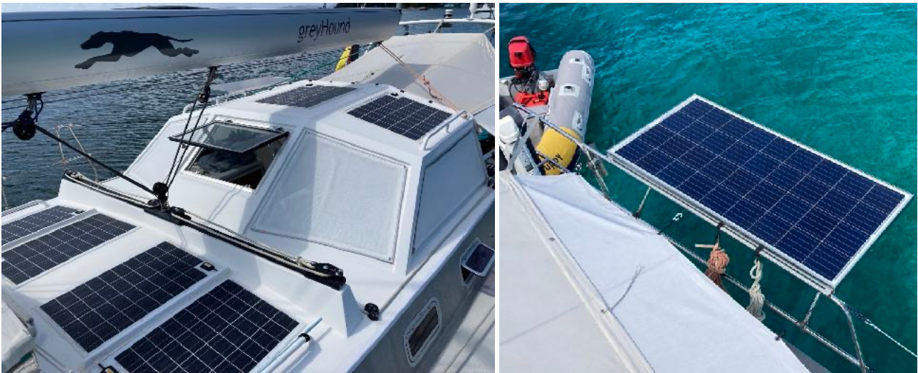
Fig. 2 left: Solar panels glued to the fixed dockhouse and the superstructure in front of the traveler right: one of the fold-out solar panels on the forward extended pushpit
